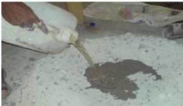
Fig- 5: Adding Alkaline solution to dry mix Fig- 6: Fresh geo-polymer concrete
