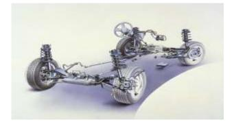
Fig 2.3: Concept of Four Wheel Steering System
