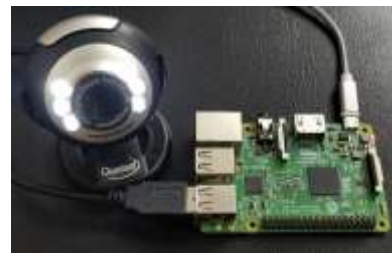
Fig-5 :Raspberry Pi 3 as the main controller and USB camera for face detection and face recognition.
