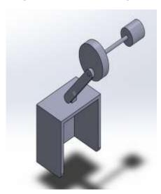
Fig -7: Assembly of Cap, Connecting Rod, Crank and Motor
