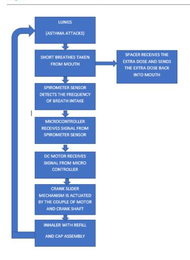
Fig -1: Block Diagram
