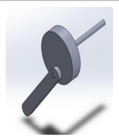
Fig -6: Crank and Connecting Rod
