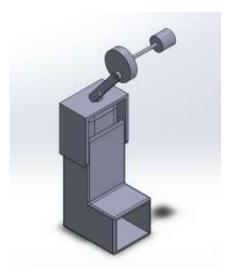
Fig - 8: Final Assembly of Automatic Asthma Inhaler
