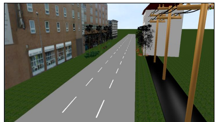
Fig.5: Study section modelled in VISSIM
