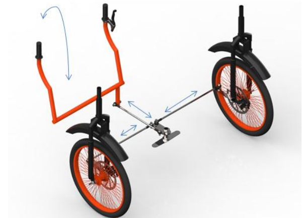
Fig-4: Steering System - Overall Geometry
