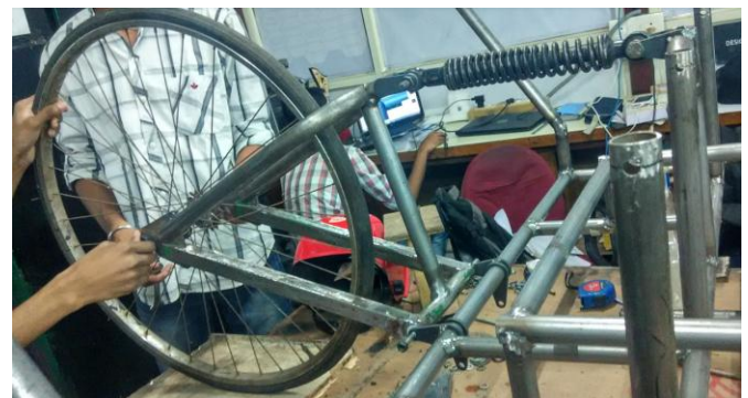
Fig-8: Single Pivot Point Rear Suspension - Manufactured
