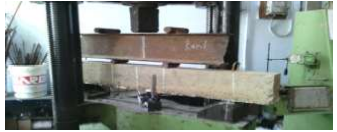
Fig -1: Universal Testing Machine (UTM) 600 kN capacity
