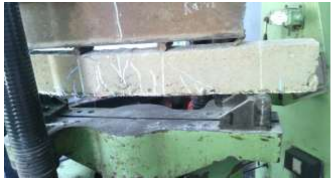
Fig -2: Cracks in control beam
