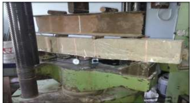
Fig -3: Crack pattern in beam with BFRP sheet
