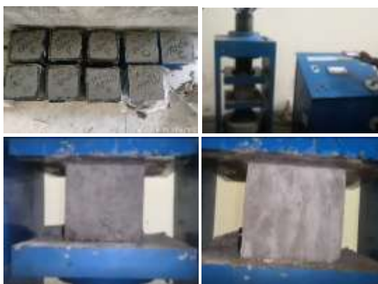
Fig -3: C. S. Test Procedure in CTM
