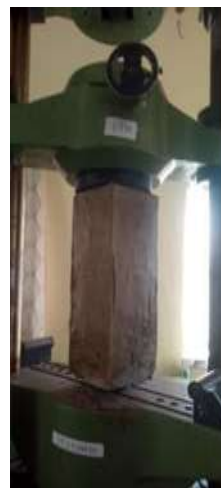
Fig-12 – basalt fibre wrapped column in UTM
