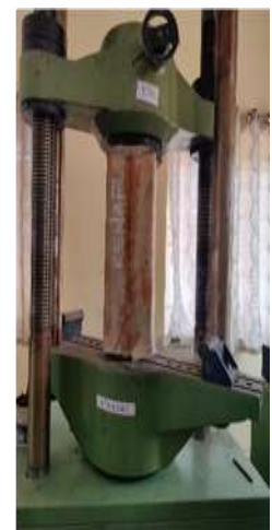
Fig-12 – basalt fibre wrapped column in UTM
