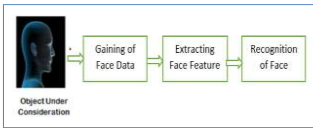
Fig. 1. Block Diagram of the face recognition system
