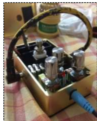
Fig 15. Distortion Effects Pedal after assembling and testing Stomp Box V6 (photo captured while making PC – self)
