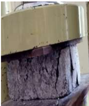
Fig.5 TESTING OF PAVER BLOCKS
