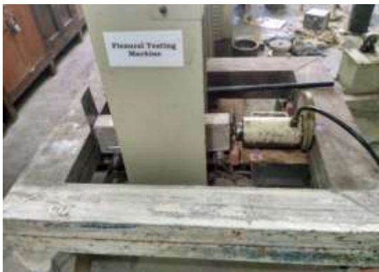
Fig. 2: Testing of SFRC under combined state of of flexure, compression and shear front view
