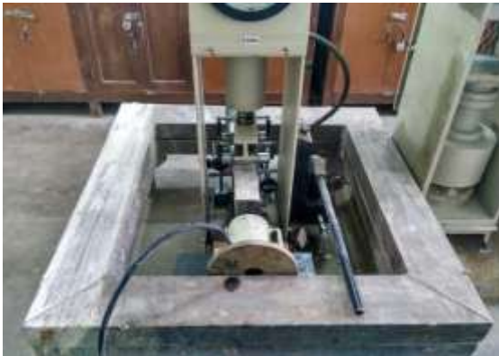
Fig. 1: Testing of SFRC under combined state of of flexure, compression and shear
