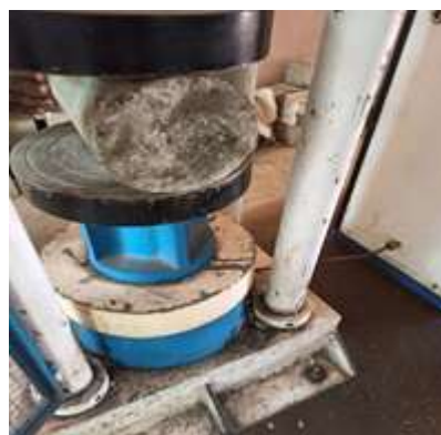
Fig -5: Split Tensile Strength Testing Arrangement
