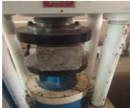
Fig -4: Compressive Strength Testing Arrangement
