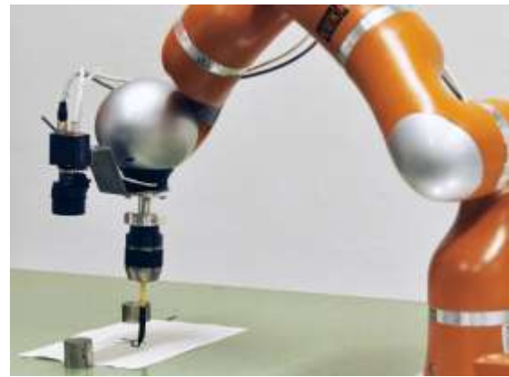
Fig. 1.0. The experimental setup consisting of a KUKA Light Weight Robot, a Prosilica GC 655C camera, and a brush[16].
