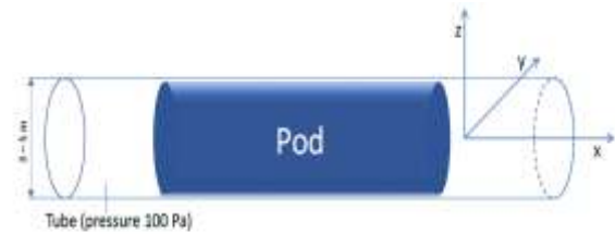
Figure 1: Operating principle of Hyperloop: a transport container („pod“) moves in a tube in near-vacuum (100 Pa)
