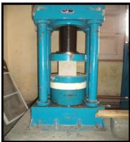
Fig 2 Compressive strength test set up
