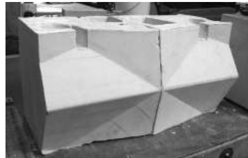
Fig- 1: Breathe brick with faceted surface
