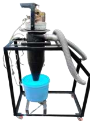
[Final Component Assembly of Grain Transfer System]
