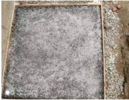
Fig 7.12 Final model of the geogrid road
