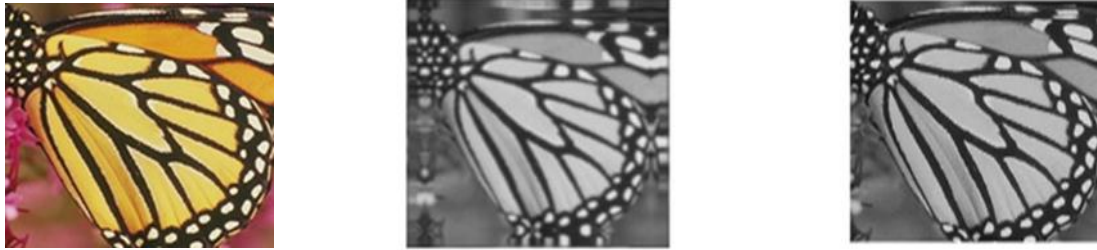
Fig2: Deblurring result for the image Butterfly blurred with 9 \times 9 filter and corrupted by noise of standard deviation \sigma=v2 . From left to right: original image blurred image, MSEPLL ( \sigma=v2 , PSNR=29.750)
