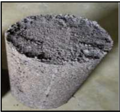
Fig-5: Ferro cement cylinder
