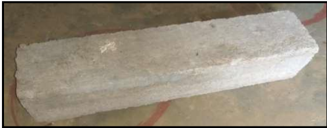
Fig-4: Ferro cement beam
