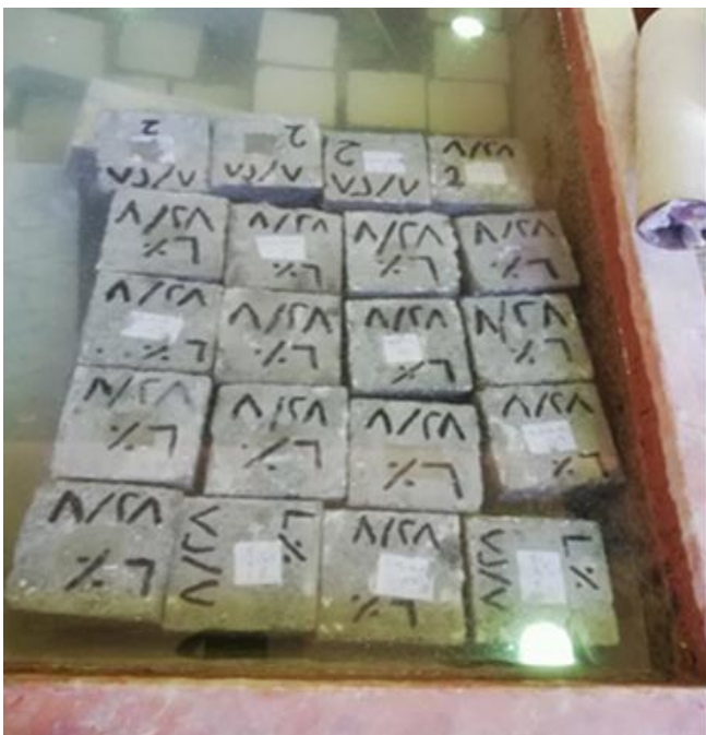
Fig -5b: Cubes (100 mm *100 mm*100mm) during curing.
