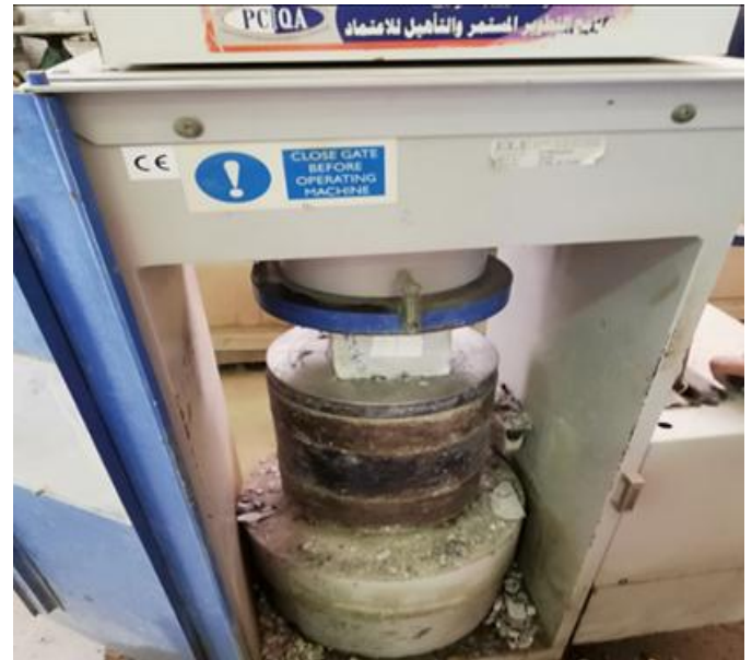
Fig -9: Cube (100 mm * 100 mm * 100 mm) during compressive strength test.
