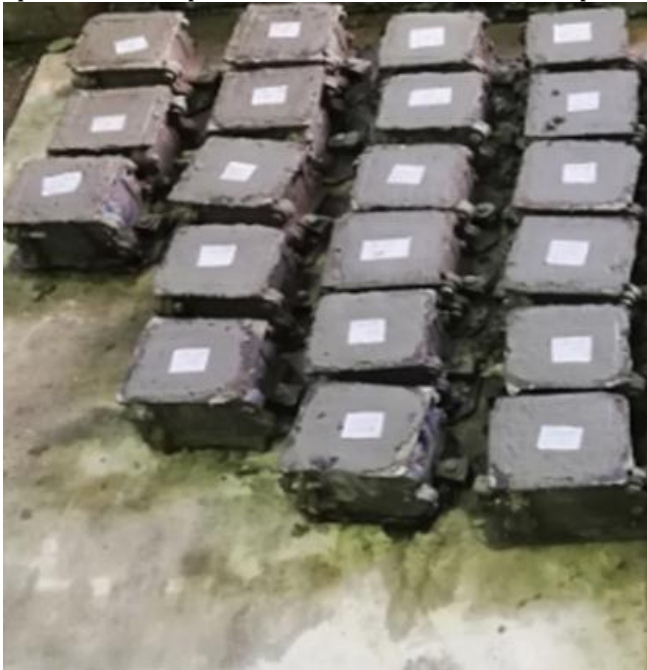
Fig -5a: Cubes (100 mm *100 mm*100mm) during casting.
