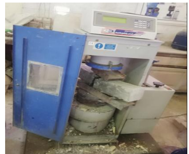
Fig -10: Beam (100 mm * 100 mm * 500 mm) during flexural strength test.
