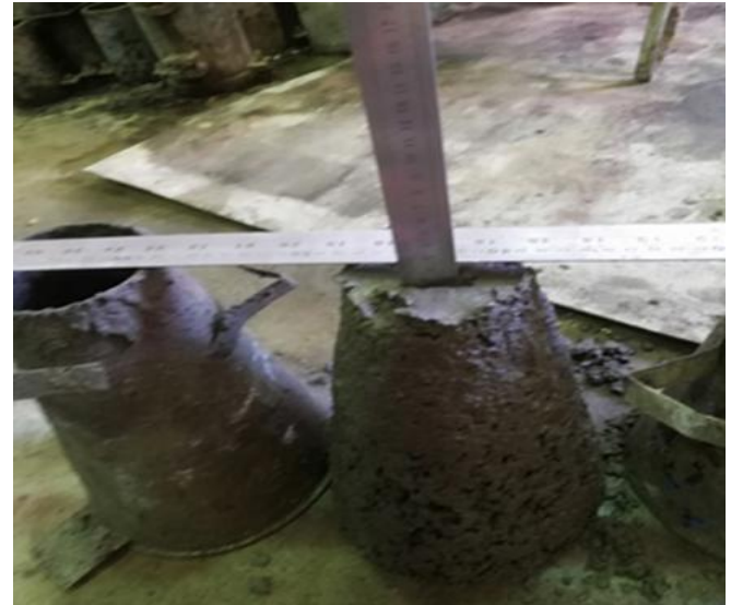
Fig -7: Slump Test.
