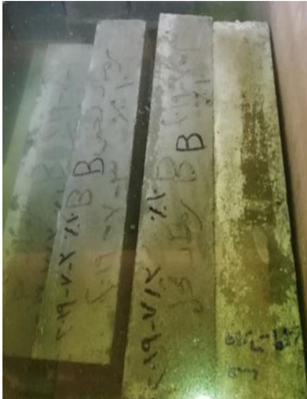
Fig -6b: Beams (100 mm *100 mm*500mm) during curing.
