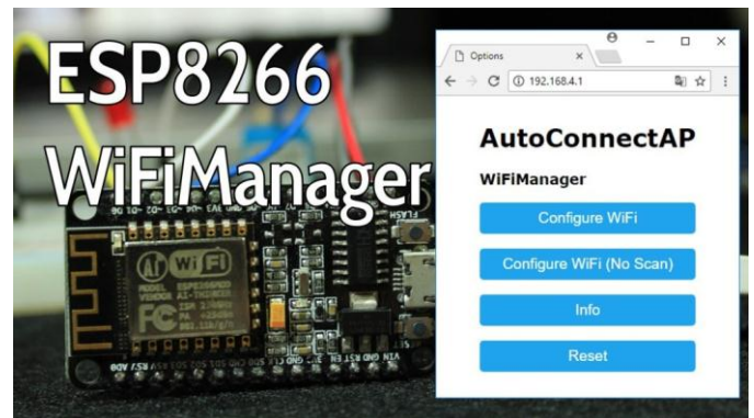
Fig: Wifi Manager with nodeMCU ESP8266
