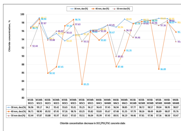
Fig.8 Cl - penetration in pre-conditioned control/IC slabs
