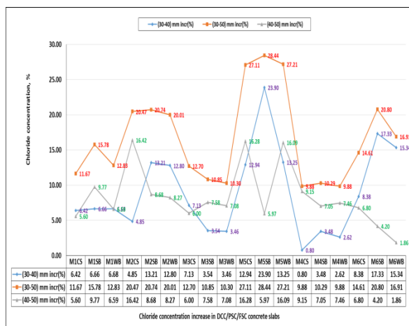
Fig.5 Cl- penetration in pre-conditioned control/IC slabs
