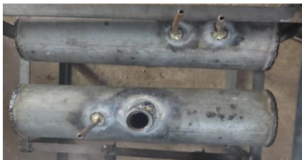
Fig-3.7: Air and tack coat storage tanks
