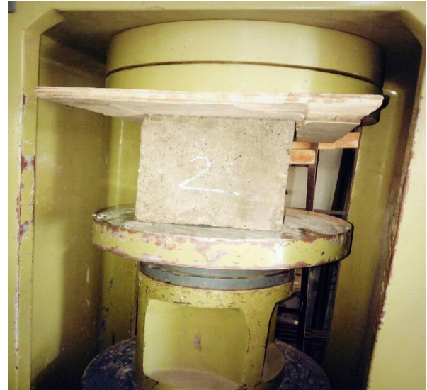
Fig.1. Setup for Compressive Strength Test
