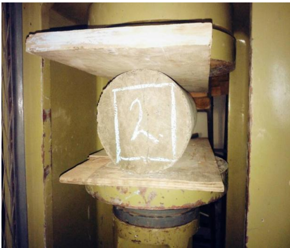
Fig.2. Setup for Split Tensile Test
