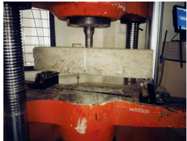
Fig.3. Setup for Flexural Test
