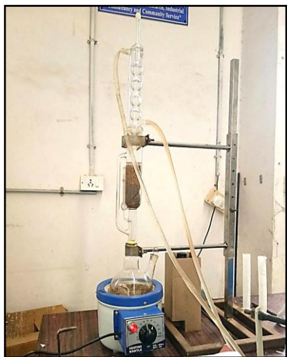
Fig. 1: Experimental set-up for extraction of oil from custard apple seeds.
