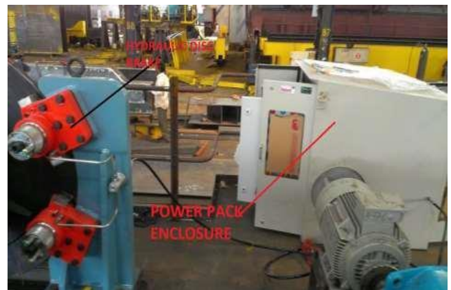
Fig - 4: Safety Braking System
