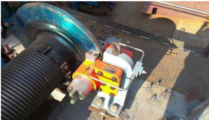
Fig -5: Safety Braking System
