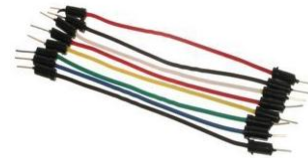
Fig. -4: Connecting Wires
