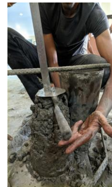
Fig 2: Slump cone conduct
