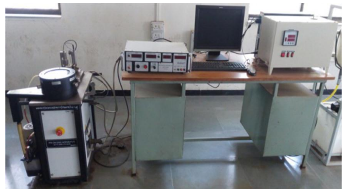
Figure - 2: Pin-on disc sliding wear testing machine with integrated system.
