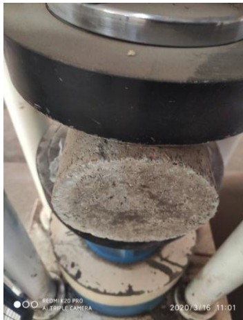
Fig -4: Cylinder Testing
