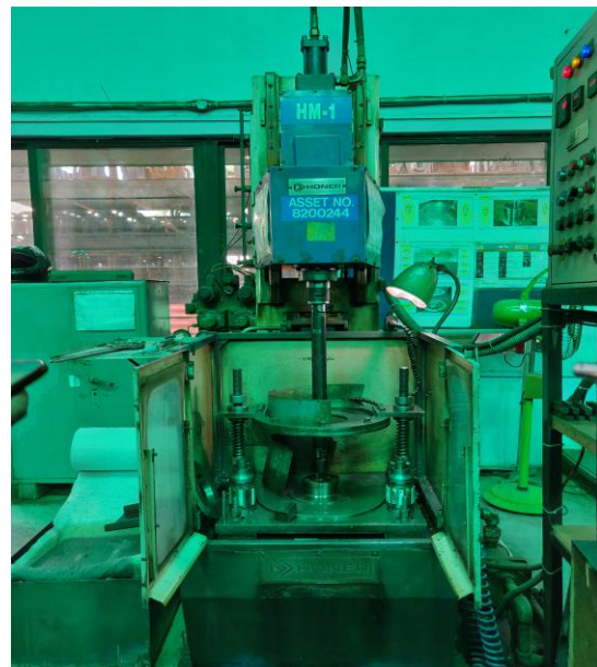
Fig - 4: DHV-100 Vertical Honing Machine
