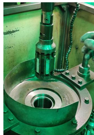
Fig - 5: Working of Honing process
