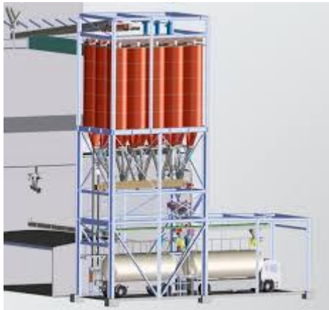
Fig. 2 Truck load silo
