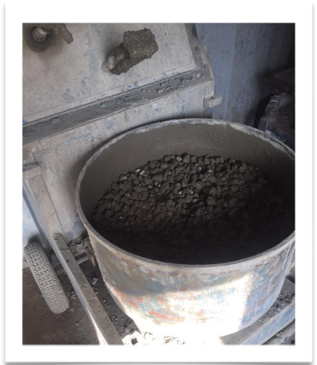
Fig -3: Mechanical Mixer
