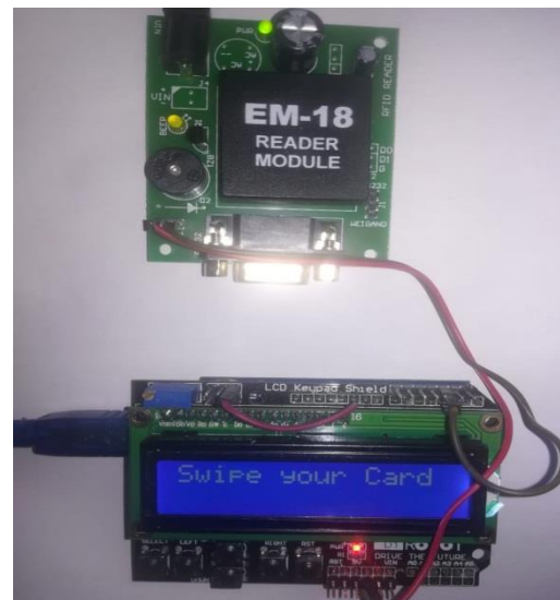
Figure-3b: System asking user to swipe the card on the card reader
