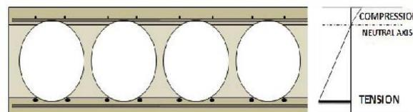
This is not the last of the benefits of the Bubble deck slab floor system: due to the lower weight of the ground system itself, also the supporting constructions such as columns and foundations can be less heavy. This can result eventually during a total weight or material saving on the building construction of up to 50 %. Since the load of the structure reduced, this sort of structure can useful to scale back earthquake damage.
