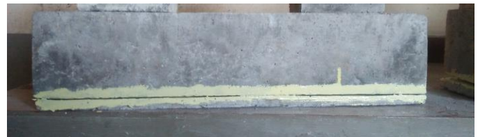
Fig 3.4: Beam bonded with SIFCON Laminate
