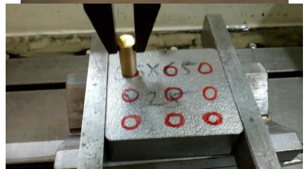
Figure: WORK PIECE SET UP IN EDM
