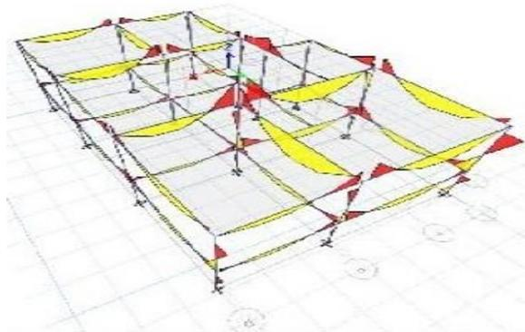
**B. Envelop Shear Force Diagram**
