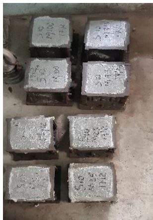
Figure.3- Casting of cubes
