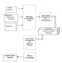
In this architecture diagram, GPS sensor, Magnetic Induction sensor and Keypad are connected a Micro controller (ATmege328) this is water data transmitter module which use the wateras Communication Medium. Similarly,
