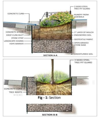
2. There are different standard sizes for Bioswale beds and they are usually filled with one tree and different types of plants and shrubs. The tree and plants are carefully chosen so they can survive on a busy City street and absorb a lot of storm water. These plants also don't mind when storm water stands for a short time in the slight depression at the center of the Bioswale.
