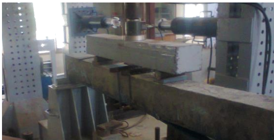
Fig: 2 Failure pattern of FRC-FWB-1
