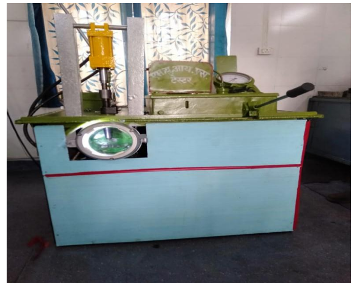
Fig 2:Hydraulic Actuated Fuel Injector Testing Machine
