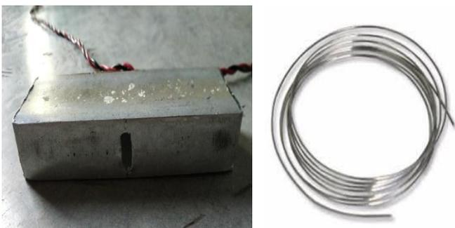
Heat sealers apply the heat and pressure to the pouch for sealing and cutting the pouch. It is work on the DC current of 5 Ampere and 12 volt supplies.
