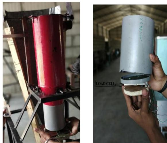
The valve plate of this valve contains the load cell which will assure the required quantity. When the controller reads the preset quantity the servo motor give motion to the valve plate and then material will falls in the packet trough the tray.
