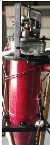
Here, Cyclone separator is used for the feeding the product into the machine. In cyclone separator there is sudden pressure drop so the dense material fall down and the dust particles exhausted from the blower side.
