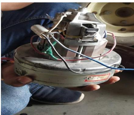
The product will sucked in the cyclone separator by creating the vacuum with the help of the blower and induction motor.
