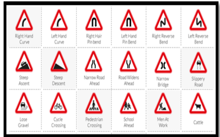
Fig-4: Warning or Cautionary Signs
