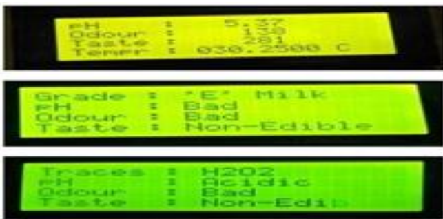
Fig. 9: Test Result of adulterated milk sample
