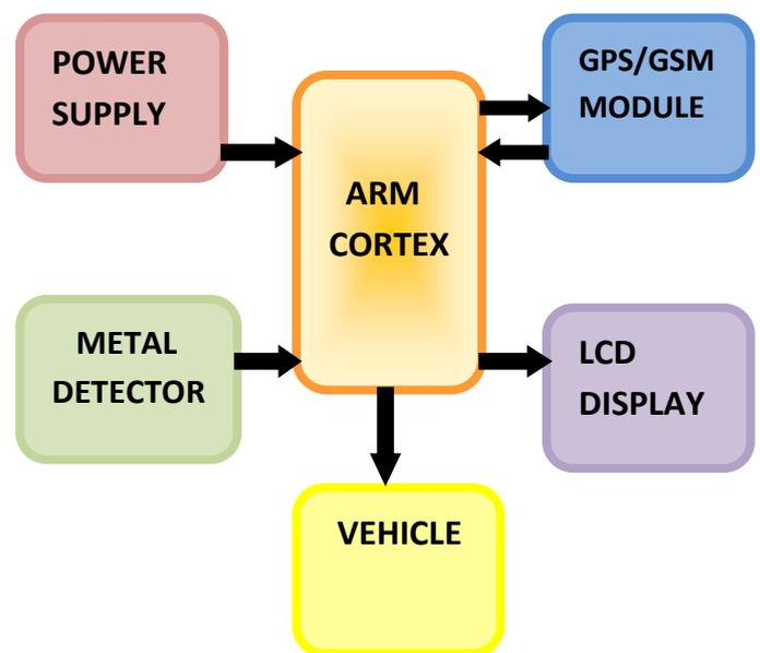
These are main components present in designing landmine detection robot:
